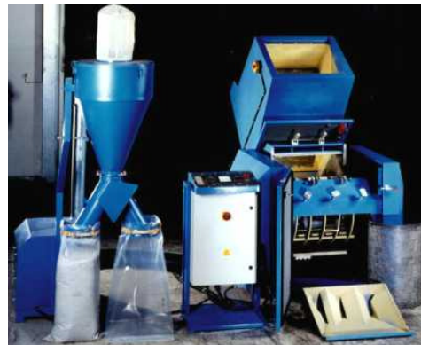
Fig. 6: HERBOLD - Blade granulator with material extraction
