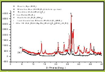
Fig 3: XRD charts of fired materials with (a) optimum slag/clay mixture (b) 0% slag
