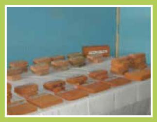
Fig 2: Fired bricks and tiles from slag/clay mixture
