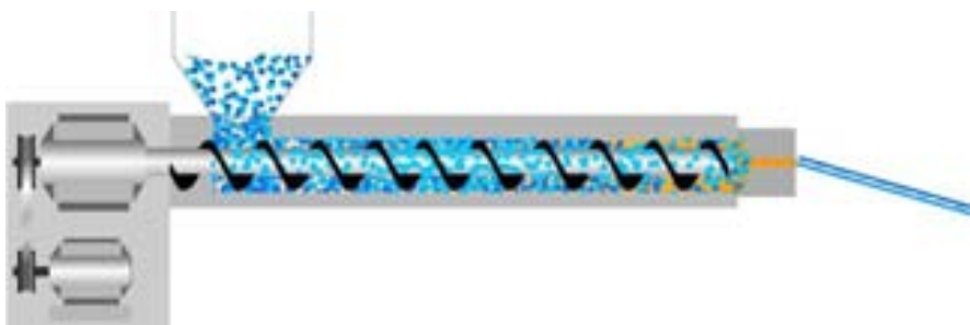
Fig. 11: Plastic profile manufacture by extrusion (source: www.anaip.es )
