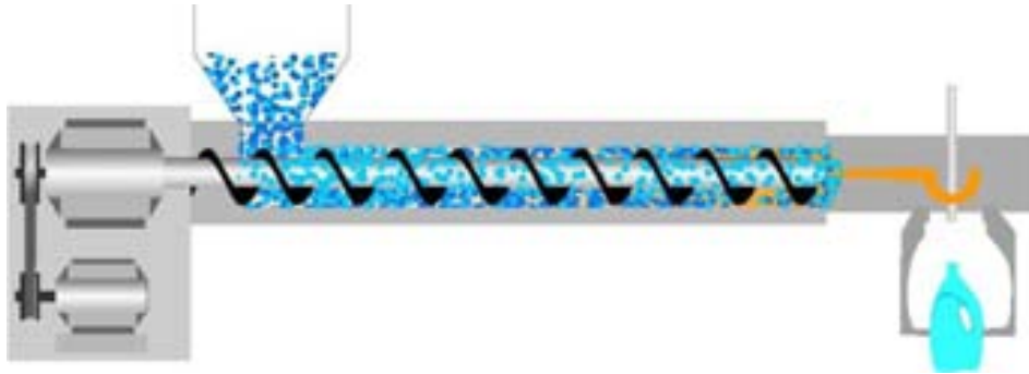
Fig. 13: Plastic bottle manufacture by injection (source: www.anaip.es)
