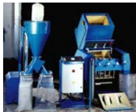
Fig. 6: HERBOLD - Blade granulator with material extraction
